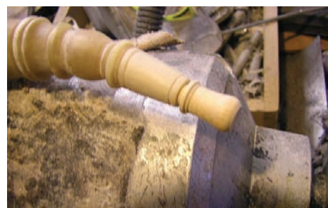
6. Stopper to protect the spout.
